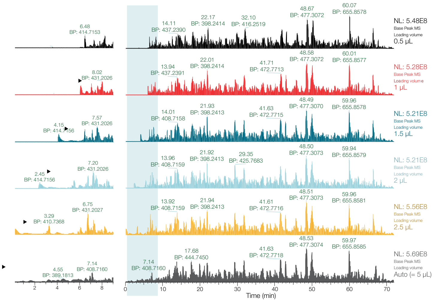
Figure 9. Base peak chromatograms obtained from the separation of 200 ng HeLa tryptic digest (1 \mu L injected) using different loading volumes. 50 cm \mu PAC Neo column, 67 min gradient. The shaded light blue section is expanded to the left.
