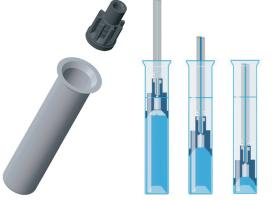
Figure 2. Autosampler sample displacement filtration.
