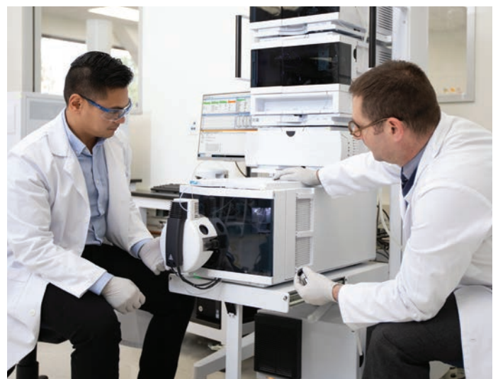
Figure 4. Ultivo utilizing the retractable bottom tray in the InfinityLab Flex Bench MS
