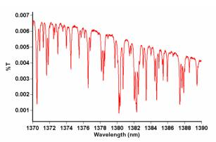
Figure 2: Water vapor transmission spectrum collected on a Cary 6000i spectrophotometer
