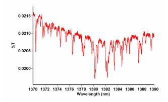
Figure 1. Water vapor transmission spectrum collected on a Cary 5000 spectrophotomer
