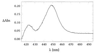
Figure 5. Baseline corrected scan of DJ4309 whole cells expressing high levels of cytochrome P-450  $\,$
