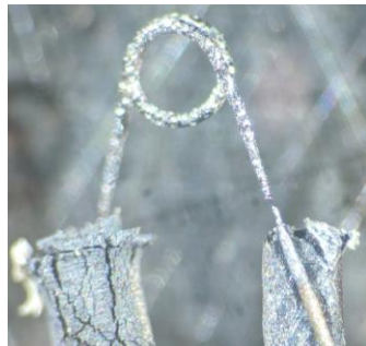
Figure 37. Two filaments that failed because of impurities in the gas supply near the ExD Cell. The white residue is an experimental coating.
