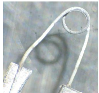
Figure 38. Example of a mechanically-damaged filament. The bent left leg pushes the loop off-center.
