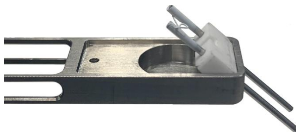
Figure 31. Sliding the filament insert into the filament cassette.
