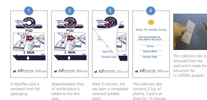
Figure 1. Noviplex plasma separation card workflow
