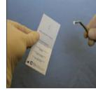
The collection disc is removed from the card and is ready for extraction for LC-MS/MS analysis.
