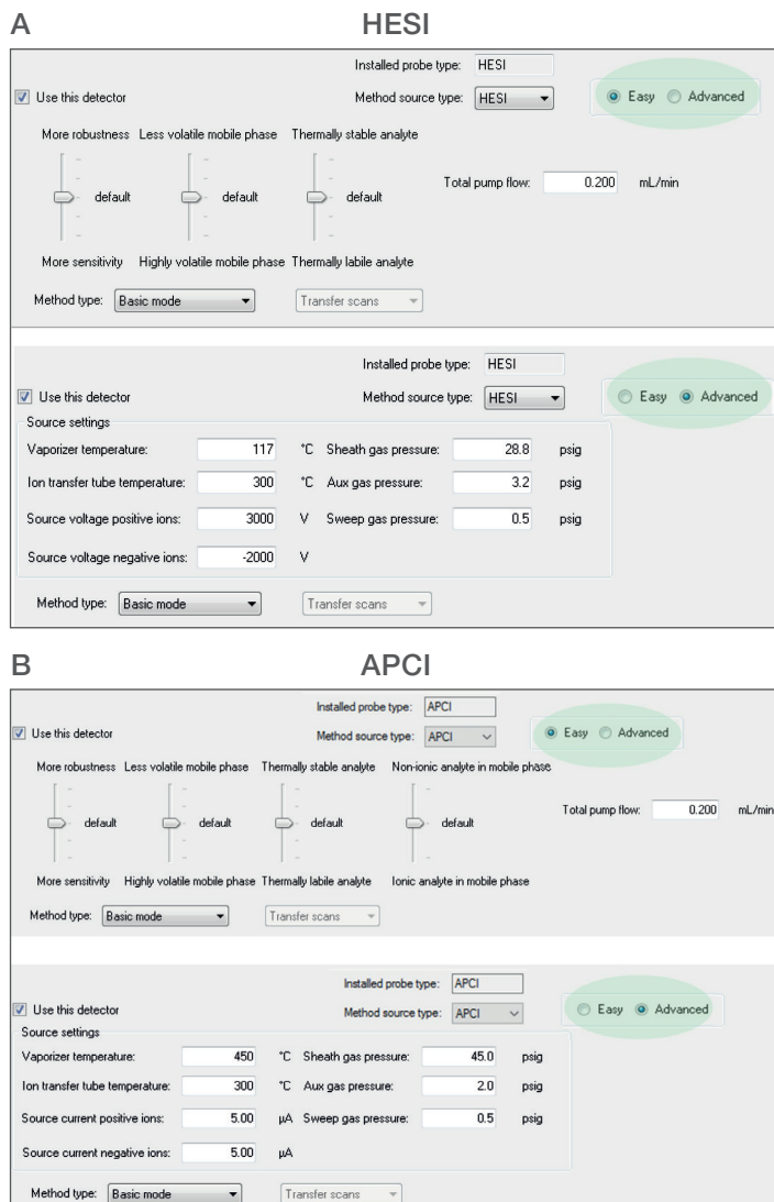
Figure 2. Automated MS method setting for heated electrospray ionization (HESI) mode (A) and APCI mode (B). With AutoSpray technology, Easy Mode enables even users without prior MS experience to easily set up their methods (top). Advanced Mode gives full access to the source parameters, enabling experienced users to further refine their methods (bottom).
