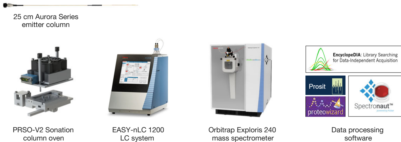
Figure 1. LC-MS setup for DIA performance evaluation
