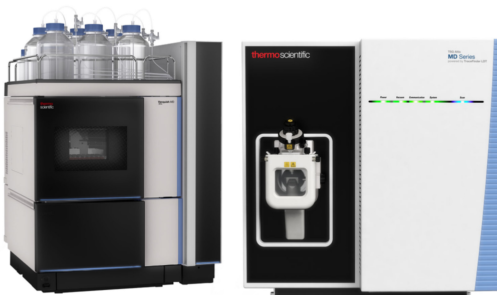
Figure 3. The developed method used a Vanquish MD UHPLC system and TSQ Altis MD mass spectrometer.
