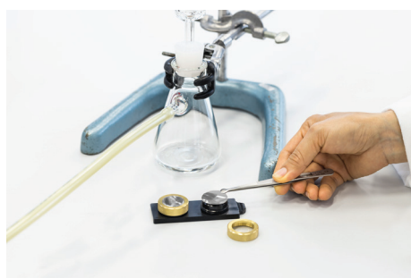
5 Place the filter on top of the raised platform
