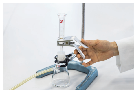
3 Secure the filtration assembly with the clamp
