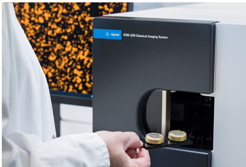
Figure 1. The Agilent 8700 LDIR Chemical Imaging System allows the high-speed routine analysis of microplastics on aluminum-coated polyester filters (25 mm, 100/0 nm coating, 0.8 µm pore size).
