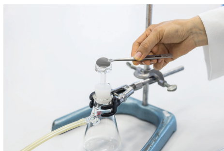
1 Place the filter using the supplied tweezers
