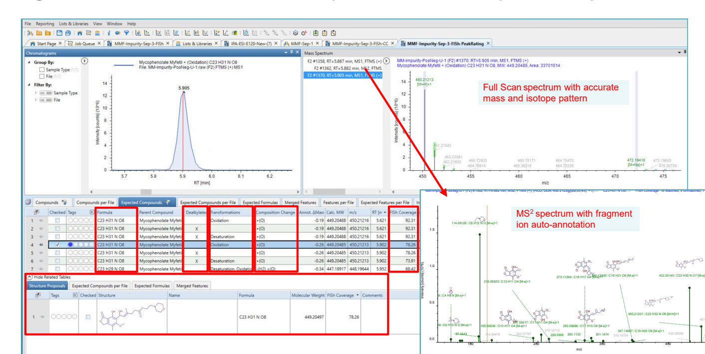
Figure 7. Full Scan and Annotated MS 2 Spectra of Identified Expected Compound
