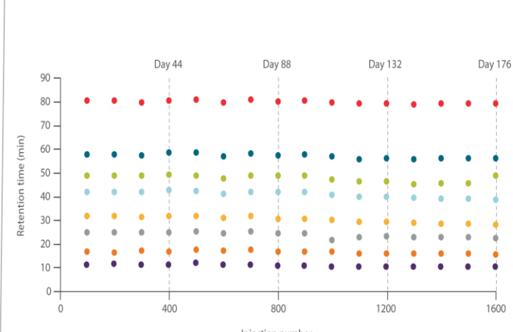
Figure 8. The retention time for 8 selected peptides from 1,600 injections of BSA protein digest over 176 days (~6 months). Each marker represents a mean of 100 injections.
