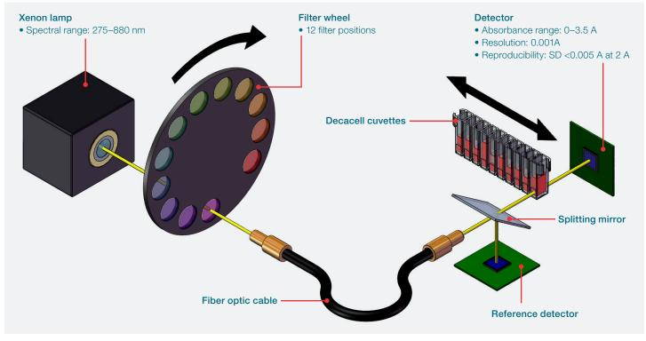
Figure 4. Gallery Discrete Analyzer-photometric measurement.
