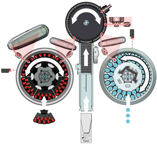
Figure 2. Direct read discrete analyzer.
