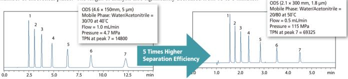
In this example, two 150 mm columns with 1.8 µm particles were connected sequentially for a total length of 300 mm. The following analytes were detected at 245 nm listed in the order of elution: Acetophenone (1), Propiophenone (2), Butyrophenone (3), Valerophenone (4), Hexanophenone (5), Heptanophenone (6), Octanophenone (7).
