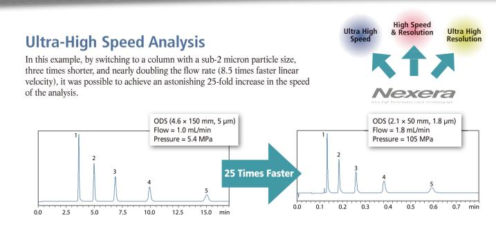
The following analytes were detected at 245 nm listed in the order of elution: Acetophenone (1), Propiophenone (2), Butyrophenone (3), Valerophenone (4), Hexanophenone (5). The Mobile Phase was Water/Acetonitrile at 45/55, 40°C.
