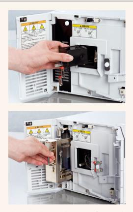
Flow Cell and Lamp replacement at front panel.
