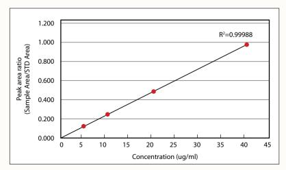
Figure 2: Linearity of peak area ratio
