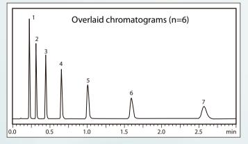
The excellent solvent delivery performance provides a high level of retention time reproducibility in both high-pressure and low-pressure gradient configurations. The figure above shows a comparison of retention time reproducibility in low-pressure and high-pressure gradient analysis. The low-pressure gradient provided excellent retention time reproducibility similar to a high-pressure gradient.
