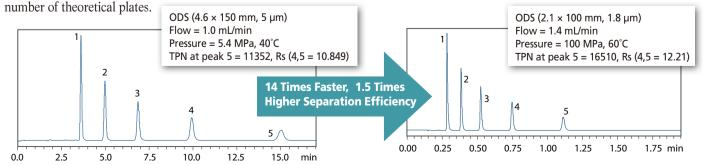
The following analytes were detected at 245 nm listed in the order of elution: Acetophenone (1), Propiophenone (2), Butyrophenone (3), Valerophenone (4), Hexanophenone (5). The Mobile Phase was Water/Acetonitrile at 45/55.
