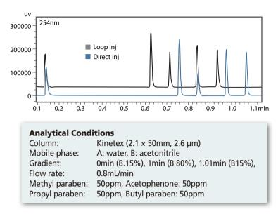
To minimize system delay, the SIL-30AC autosampler can be easily re-configured by the user to provide the absolute lowest system delay volume by conversion to a loop injector. As shown on the left, gradient delay time can be reduced drastically using loop injection. The combination of loop injection and the MiRC small-volume mixer supports ultra-fast gradients without gradient delay.
