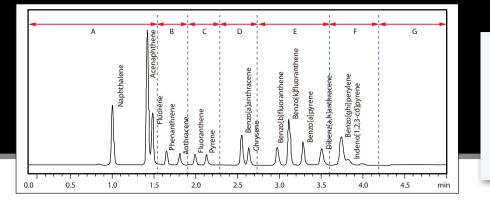
**Time-programmed wavelength switching** Ex; 270 nm, Em; 330 nm Ex; 250 nm, Em; 370 nm Ex; 330 nm, Em; 430 nm Ex; 270 nm, Em; 390 nm Ex; 290 nm, Em; 430 nm Ex; 370 nm, Em; 460 nm Ex; 270 nm, Em; 330 nm
