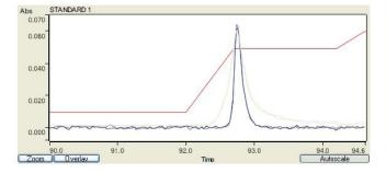
Figure 3. Temperature Profile for 0.0483 µmol/L Pb in blood standard.
