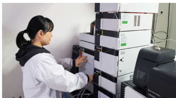
Photo: Customer of Institute for Food and Drugs Control use LCMS-8050 to detect NDMA in metformin
