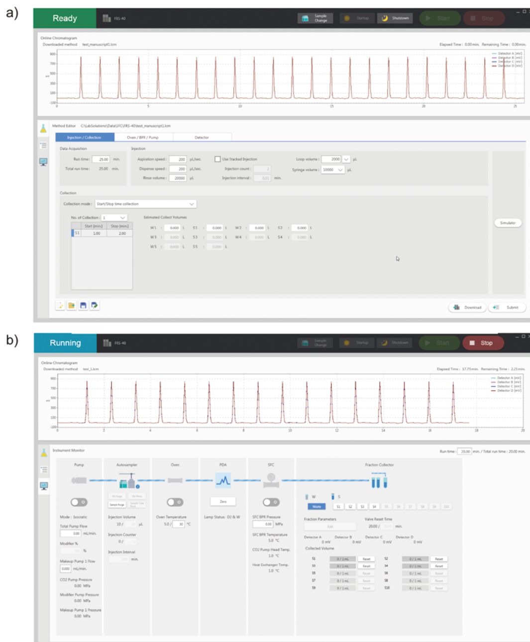
Figure 3. Snapshots from the newly developed PrepSolution software including (a) method editor and (b) instrument monitor. Data viewer is not shown.
