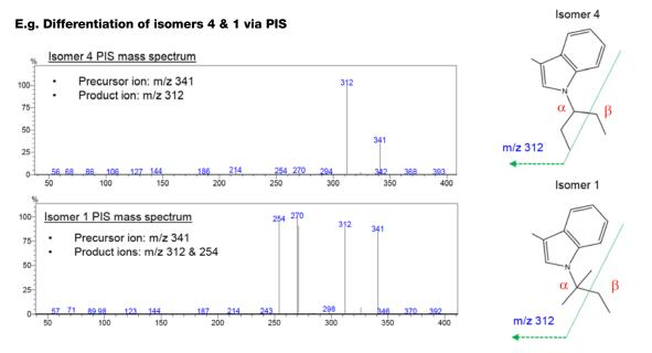
After the Ca-C<sub>b</sub> bond cleavage, stability of the resulting carbocation resulted in different product ions, i.e. distinctive PIS mass spectra.
