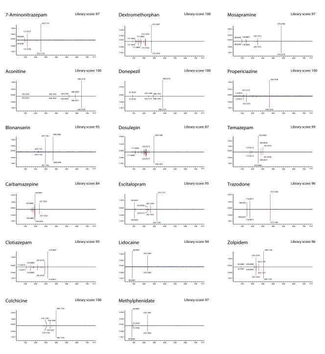
Fig. 2. (Top) MS/MS Spectra and Library Scores of Drugs (500 ng/mL) in Human Whole Blood Acquired Using *iDIA* and (Bottom) MS/MS Spectra of Standard Substances of Drugs Acquired by LC-ESI-Q-TOFMS
