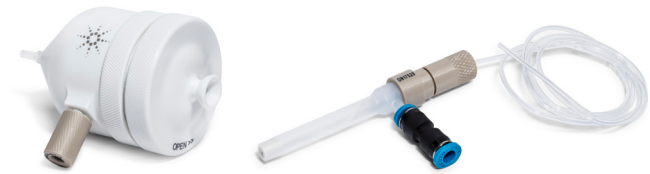
Figure 4. The Agilent inert spray chamber and OneNeb nebulizer are ideal for the analysis of samples digested with HF.
