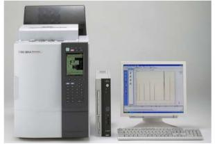
Shimadzu GC-2014 Gas Chromatograph
