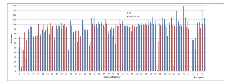
*Figure 2. Full suite of analytes from US EPA Method 8270 recovered from spiked reagent using Liquid-Liquid extraction (blue) compared to the One-Pass system (red)*
