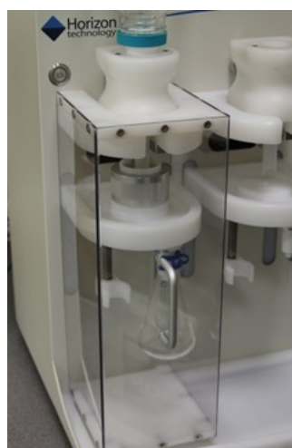
Figure 1. Vapor Shield on station 1 of the SPE-DEX 5000.
