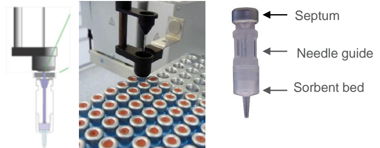
Figure 2. Cartridge needle transport and ITSP \mu SPE cartridges
