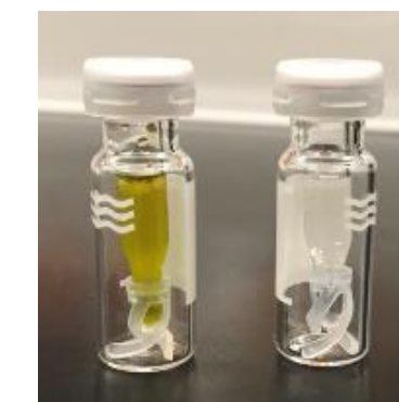
Figure 3. Leek extract without clean-up and after \mu SPE clean-up
