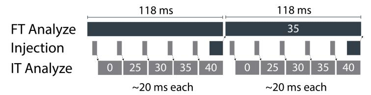
Figure 4. Pipelining of the ion trap scans for assisted collision energy determination with 60K FTMS2s. The five ion trap injections and analyses can occur during the preceding FT transient period and are used to calculate the optimal energy for the next FT injection and analysis step.
