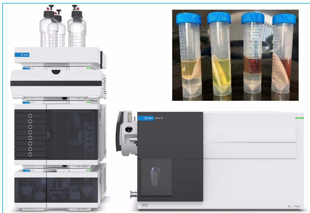
Figure 1: 1290 Infinity II, 6470 LC/TQ, Samples in PP tubes (inset)
