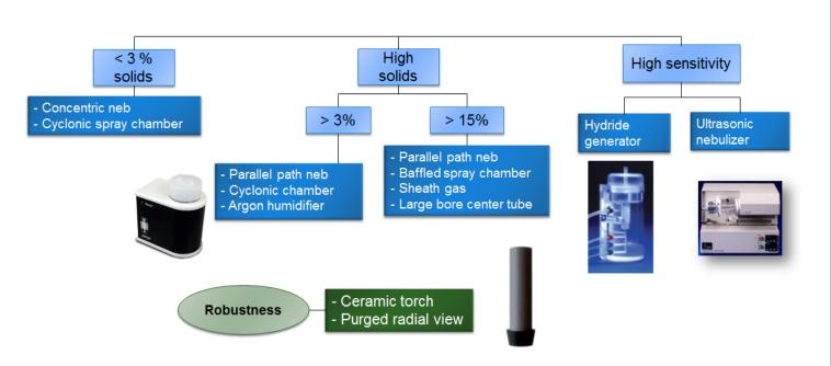
When it comes to particles in solution, nebulizers can typically handle particle sizes of up to one third of the capillary diameter before blockage occurs. When aiming for high sensitivity of some elements, an ultrasonic nebulizer or a hydride generator may be used to improve detection capability of the instrumentation.
