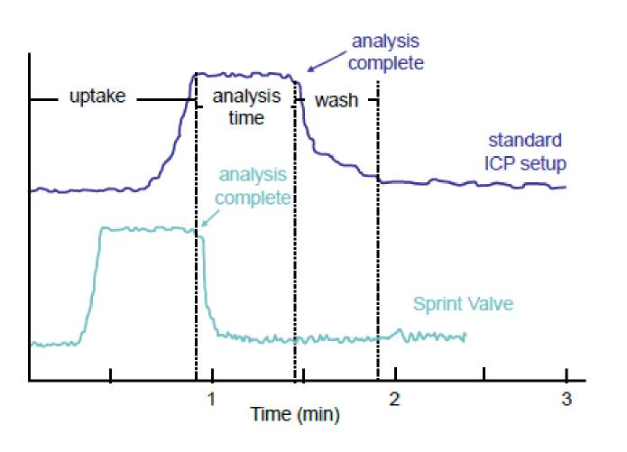
Figure 5. Total analysis time with and without Sprint Valve.
