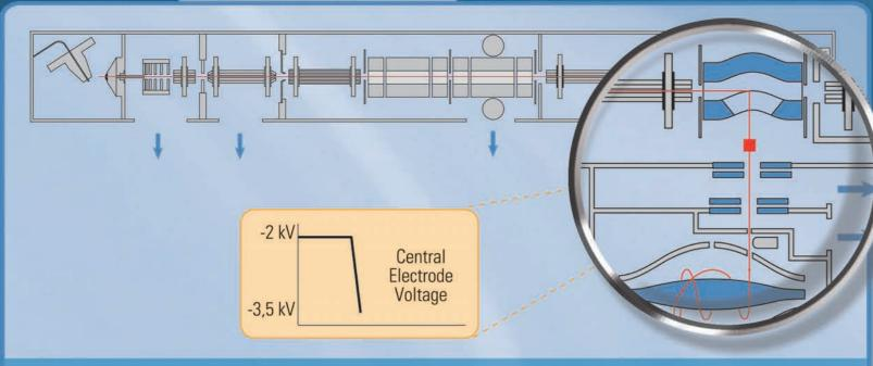
As the ions are entering the Orbitrap analyzer, the voltage on the central electrode increases and forces the ion packets into circling around the electrode. The Orbitrap, and voltages on the Orbitrap start to change.
