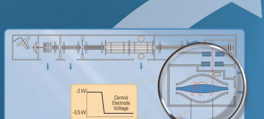
The ions entered the Orbitraps lightly off axis, and keep oscillating along the central electrode (left-right). The image current is recorded on the outer split electrodes. The signals are amplified and transformed into a frequency spectrum by fast Fourier Transformation which is finally converted into a mass spectrum.
