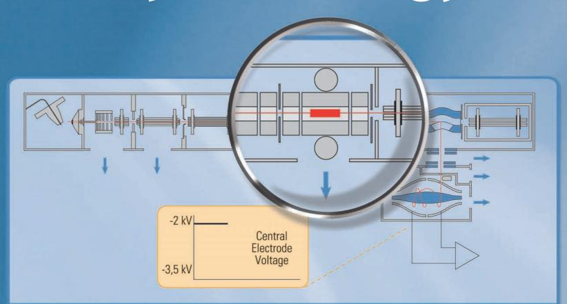
1 • Ions are injected from the ion source and trapped in the linear ion trap. Ions of interest can be isolated and fragmented in the linear ion trap, and even scanned out and detected by an independent set of detectors.
