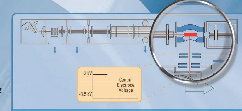
To obtain high accuracy measurements, the ions are axially ejected from the linear trap into the C-Trap where they are captured again and 'cooled' by collisions with nitrogen gas.
