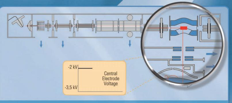
The ions are squeezed into a smaller cloud within the C-Trap ready for injection into the Orbitrap.
