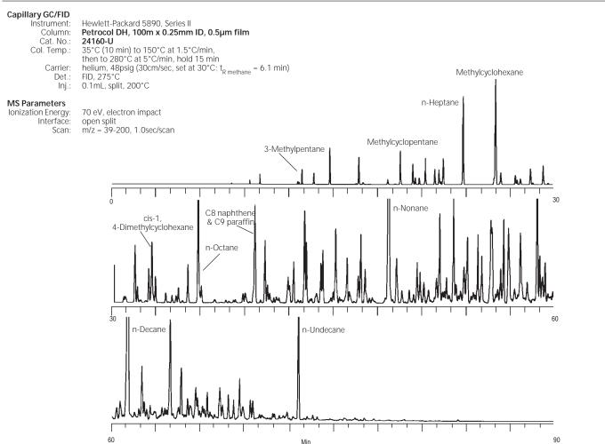
The temperature programming and linear velocity (pressure) parameters chosen are known to be suitable for a wide range of petroleum stream samples encountered by Consolidated Sciences. The analysis is isobaric, although pressure programming could be used. The head pressure used allows good separation of early eluting components and reasonable linear velocity over a wide temperature range.
