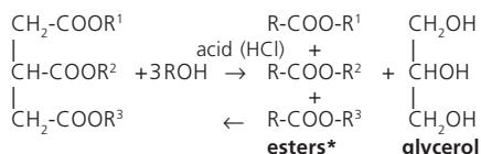
Transesterification is an equilibrium reaction. The stoichiometry of the reaction dictates that for each mole of lipid to be completely derivatized there must be 3 moles of alcohol but, in fact, it is necessary to use an excess of alcohol in the reaction mixture, or to remove one of the reaction products, to drive the reaction to the right. When the second option is employed, the reaction can go to completion.
