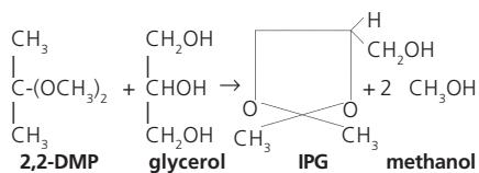
To ensure complete conversion of the lipid, the amount of 2,2-DMP used should be a molar excess of the total glycerol expected from the reaction.
