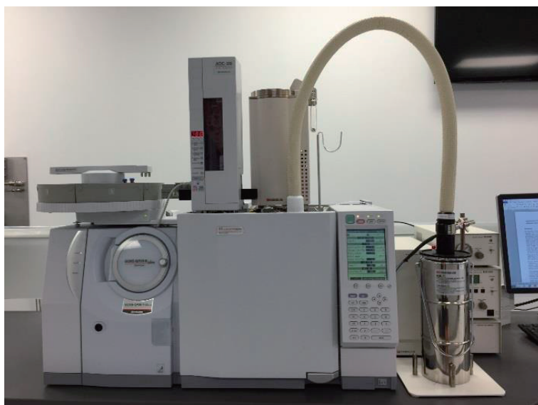
Figure 1. Frontier Multi-Shot EGA/PY-3030D pyrolyzer and AS-1020E Auto-Shot sampler installed on the Shimadzu GCMS-QP2010 Ultra
