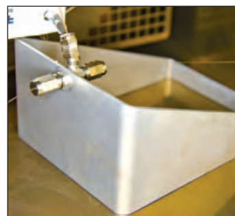
Figure 2. Splitter device holder inside the column oven (SGE)
