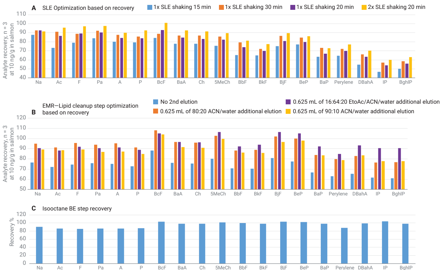
Figure 3. Sample preparation method optimization based on PAH recovery for the solid/liquid extraction step (A), EMR-Lipid cleanup step (B), and isooctane back extraction (C).
