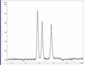
Figure 2: 2.5 uL liquid injection of 100 ppb acetonitrile and 100 ppb propionitrile diluted in MTBE
