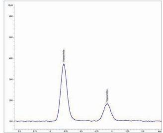
Figure 3: 2.5 uL liquid injection of 333 ppb acetonitrile and 333 ppb propionitrile diluted in TAME
