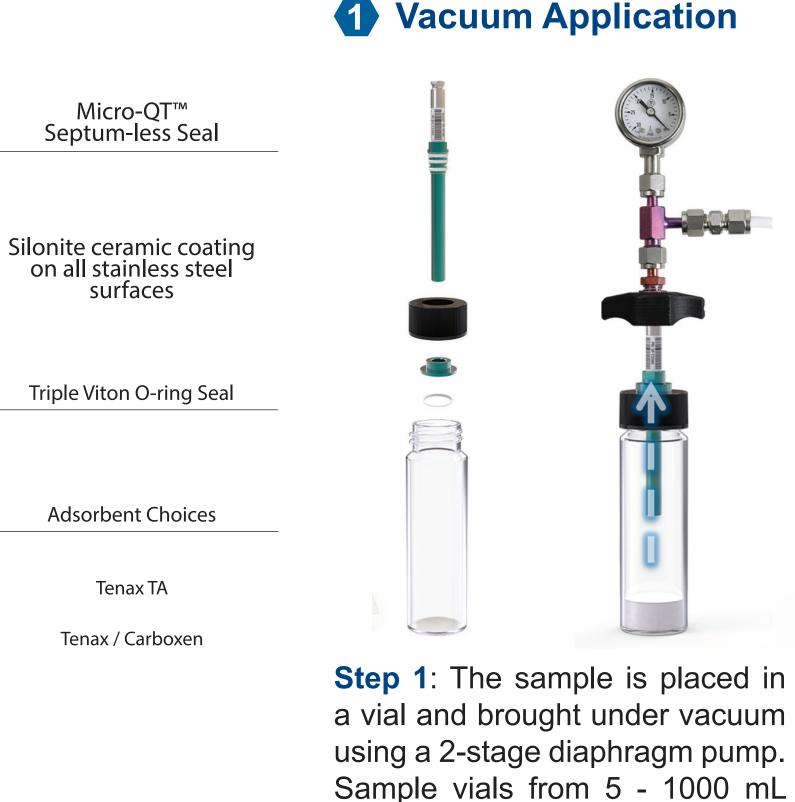
sample size is less than 1 mL. Schematic of the Headspace Sorbent Pen (HSP), showing the Micro-QT vacuum seal and the internal sorbent bed. The HSP can be packed with a variety of sorbents, including multi-component beds of varying physical properties. For the purposes of this work, ~80 mg of Tenax TA (35/60 mesh)
