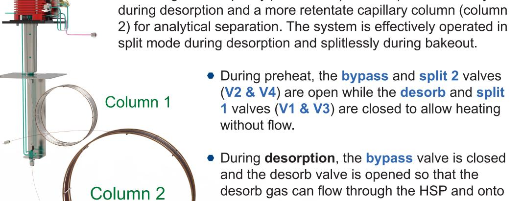
During bakeout, the split 1 valve is opened and the **split 2** valve is closed to allow SVOCs to pass splitlessly onto the analytical column.
