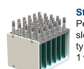
Step 4: Extracted Sorbent Pens are placed in isolation sleeves, where they can typically be stored for up to 1 week prior to TD-GC-MS.
