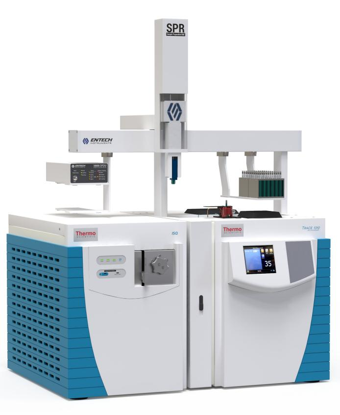
Sorbent Pen Thermal Desorption (SPDU) and Sample Preparation Rail (SPR) positioned on top of a Thermo GC-MS. The SPR transfers Sorbent Pens between the SPDU and air-tight isolation sleeves. The SPDU is connected directly to a capillary GC column held within the GC oven, which helps to minimize the flow path and mitigate analyte loss and/or carryover. Important optimization parameters include flow rate, preheat temperature & duration, desorption temperature & duration, and bakeout temperature
