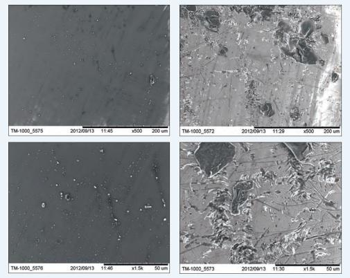
Figure 3: Comparison of new and re-washed glass vial surfaces
