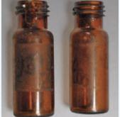
Figure 2c: Remains of identification patches on amber vials after re-washing
