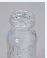
Figure 2b: Typical re-wash screw thread damage
