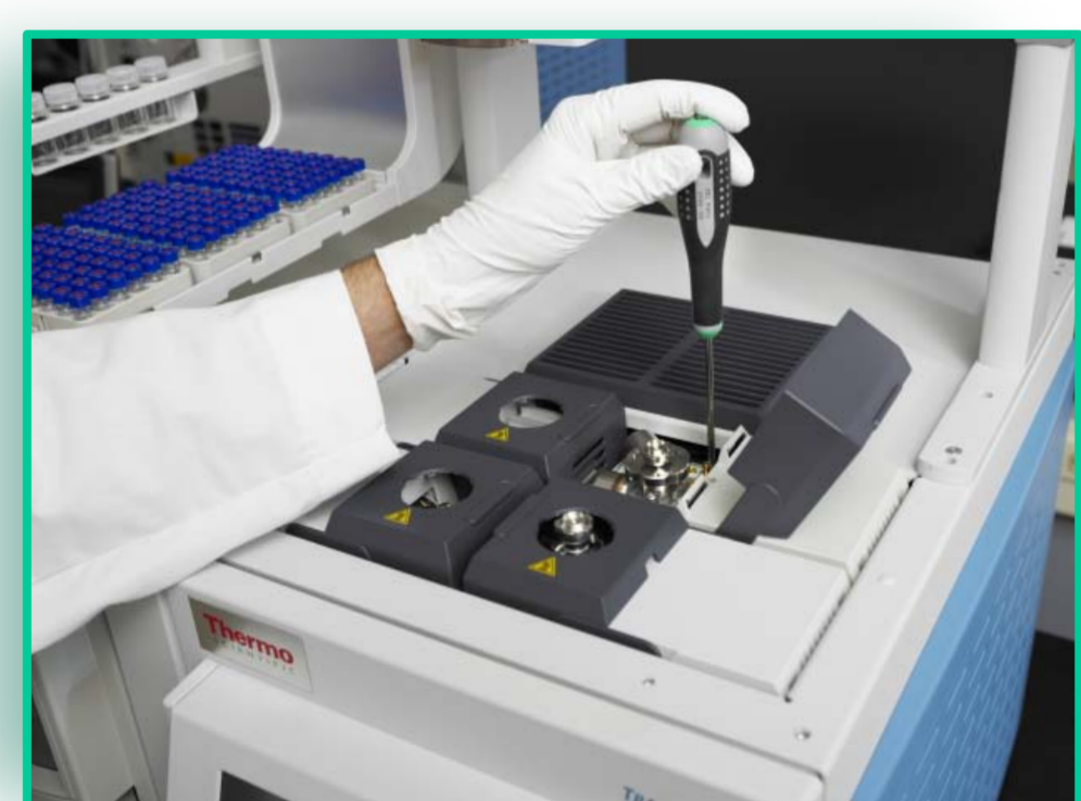
FIGURE 1. TRACE 1300 Series GC Modularity with user-installable modules
