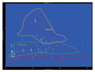
Figure 2. GCxGC chromatogram displaying the TIC and the Classification regions for the alkanes, aldehydes, and alcohols. Notice only peaks within the Classification regions are displayed with black peak markers. The use of Classifications not only aids in compound identification but also provides the analyst with a more efficient way to view the processed data.
