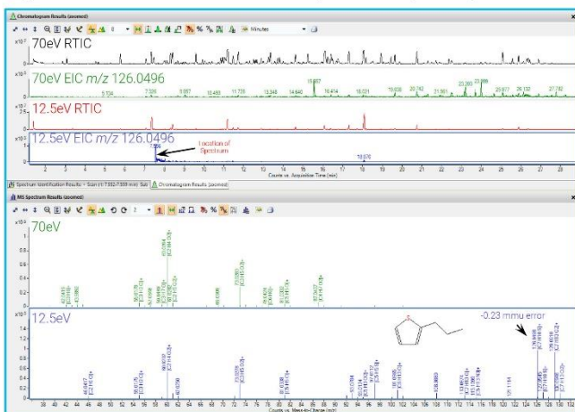
Figure 4: Comparison of 70eV and 12.5eV for a co-eluting component.
