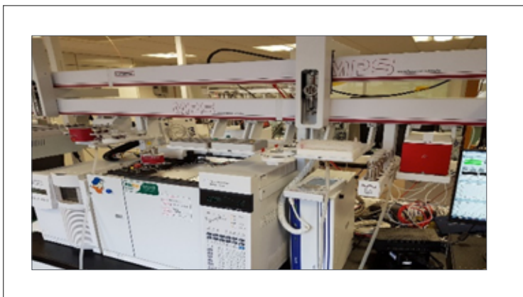
Figure 1: Agilent 7890B/5975B GC/MS used for this analysis. The GERSTEL MPS XT has been equipped with an Agitator and SPME capabilities.
