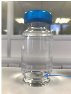
Figure 3 – High recovery vial with low volume of the dichloromethane present at the bottom of the vial
