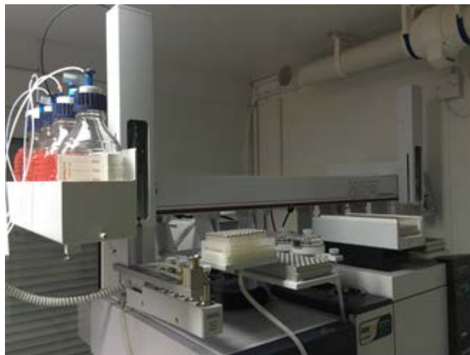
Figure 2. Agilent 7000 GC/MS/MS and Dual Head GERSTEL MPS with on-line ITSP, SFS and flow cell at Affinity Water's treatment works.
