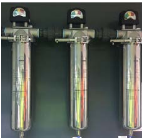
Figure 5. On-line inlet Agilent 7000 GC-Triple Quadrupole filtration
