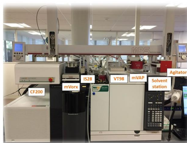
Figure 1: GERSTEL Dual Head MPS for fully automated MOX-TMS derivatisation for metabolomics applications
