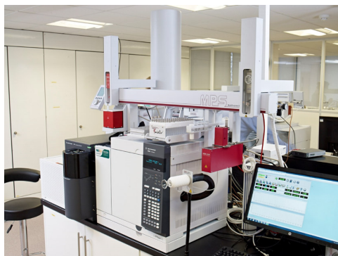
Figure 2 MultiFlex GC/Q-TOF with DHS and Static Headspace with Odour port at Anatune.
