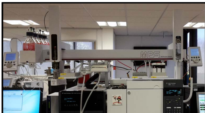
Figure 1: Gerstel Dual Head MPS with Agilent GC 7890B coupled to MS QQ 7010
