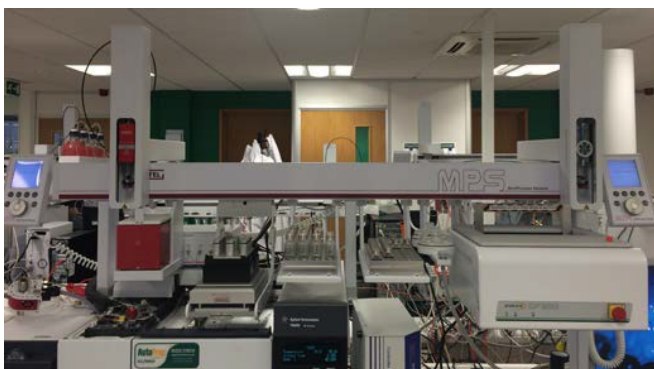
Figure 1 – GERSTEL Dual Head, mVortex and Centrifuge with Agilent GC-MS (5977) at Anatune
