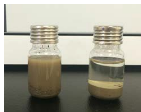
Figure 2 – Soil samples before and after centrifugation
