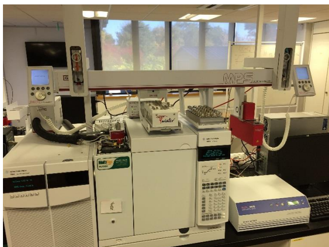
Figure 1: DHS-GC/MS MVM with the TDU/CIS injector
