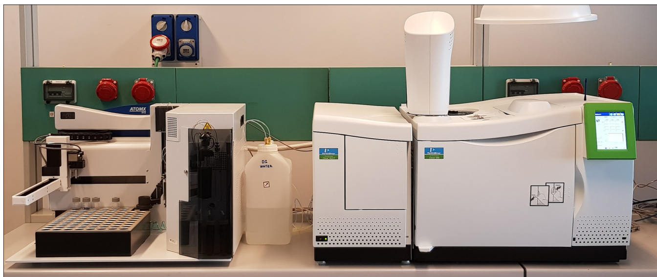
Figure 1. System P&T with Clarus SQ 8 GC/MS.
