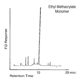
Pyrolysis of Polyethyl Methacrylate, 600°C for 10 seconds
