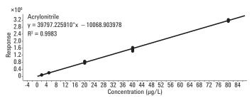
**Figure 2.** Calibration curve for acrylonitrile gave a correlation coefficient of 0.998 for five levels, ranging from 2  $\mu$ g to 80  $\mu$ g.
