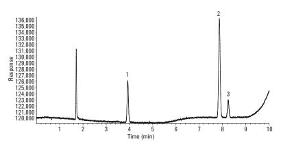
Figure 4. Acrolein (1), acrylonitrile (2), and acetonitrile (3) at 1 mg/kg eluted in under 10 minutes.
