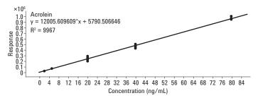
Figure 1. The calibration curve for acrolein from 2  $\mu g$  to 80  $\mu g$  gave a correlation coefficient of 0.997.
