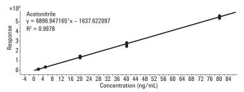
Figure 3. Acetonitrile gave a correlation coefficient of 0.998 for five calibration levels, ranging from 2  $\mu$ g to 80  $\mu$ g.
